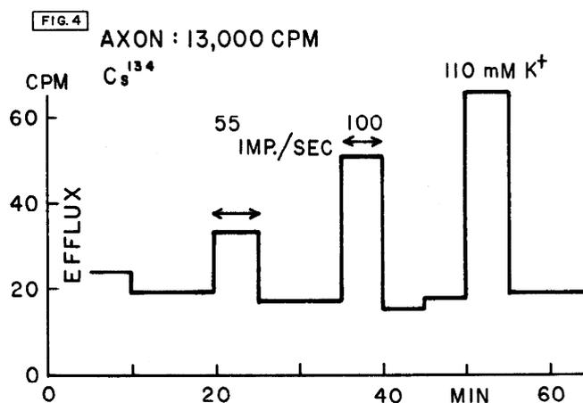
FIG. 4. Efflux of intracellular radioactive cesium during rest repetitive stimulation, and potassium depolarization; each collection period 5 min; axon diameter  $220\mu$ .
