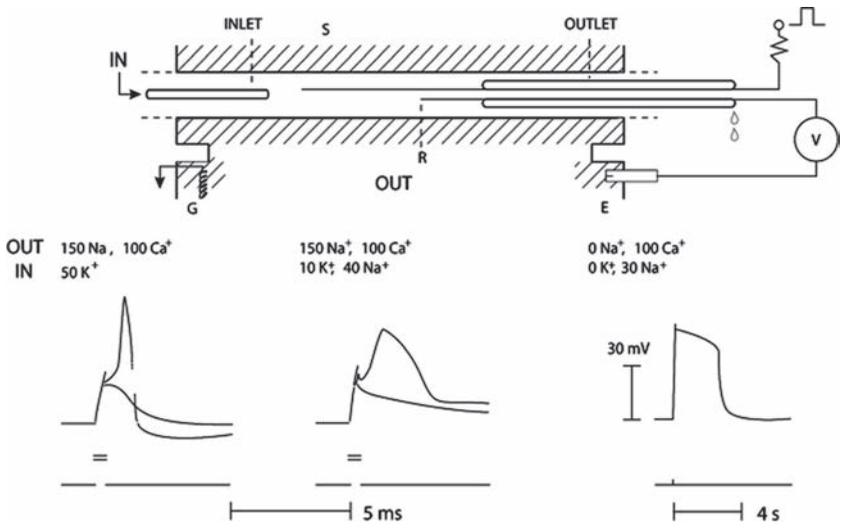
**Fig. 6** *Top:* Schematic diagram illustrating the setup for intracellular perfusion of a squid giant axon. *Bottom:* Action potentials recorded from an axon. The concentrations of the cations in the extracellular (OUT) and intracellular (IN) salt solutions are indicated (Tasaki, 1982)
