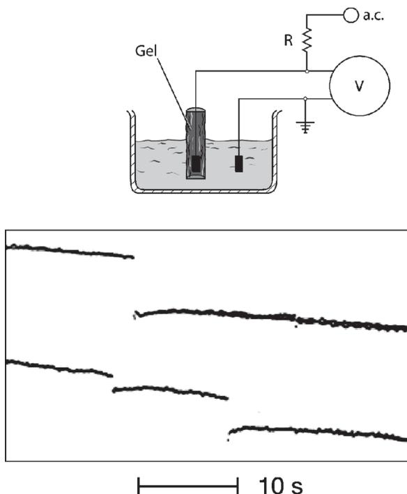
**Fig. 4** Abrupt fall of the electric impedance across the superficial layers of a compact gel rod immersed in a 100 mM NaF solution. The impedance at 1 kHz was 1.1 k $\Omega$ , and the change observed in the upper trace was about 1% initially. (Tasaki, 2005b)
