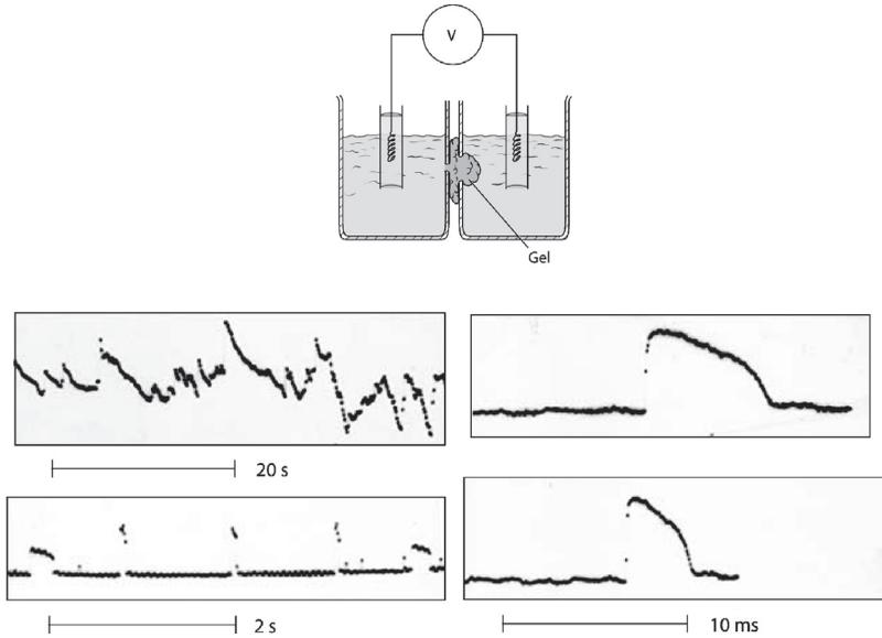
**Fig. 5** Variation of the potential difference across a compressed gel layer that were exposed to a 100 mM NaF solution on one side and to a 66 mM CaCl<sub>2</sub> solution on the other side. The amplitudes of the abrupt potential changes were between 1 and 24 mV (Tasaki, 2005b)
