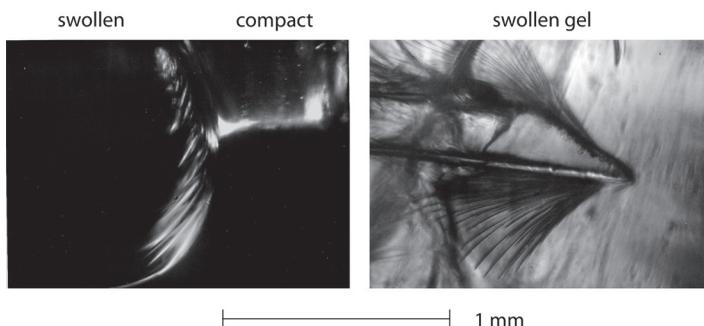
**Fig. 3** *Left*: Highly refractile bundles of polymer chains formed in the transitional zone between the compact and swollen regions of a cross-linked polyacrylate gel strand. *Right*: Bundles of polyelectrolyte chains formed inside a swollen gel by application of an electric current by use of a glass pipette containing a  $\text{CaCl}_2$  solution (Tasaki, 2005b)
