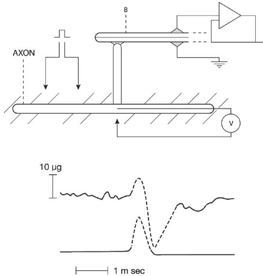
**Fig. 7** *Top*: Schematic diagram illustrating the piezoelectric device for detecting small and rapid pressure changes associated with excitation of a squid giant axon. *Bottom*: Mechanical response and action potential recorded simultaneously (Tasaki 1982)
