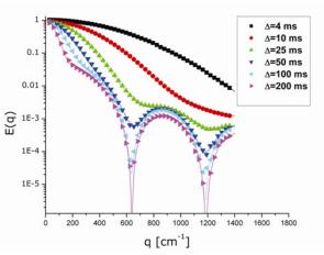
Figure 2. Varying diffusion periods in s-PFG experiments performed on a bicompartmental phantom consisting of microcapillaries with inner diameter of 19 µm in the SDC and 80 µl of water in the FDC. The gradient duration was  $\delta$ =2 ms and G<sub>max</sub>=160 g/cm. Symbols represent experimental data, while the solid lines represent the theoretical fitting to the experimental data.
