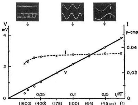
FIG. 2. Relationship between the amplitude of the membrane potential variation,  $V$ , at the site of application of sinusoidal currents of amplitude  $I$  and the frequency,  $f$ . Note that the phase difference between the two sine waves in the photographic records on the top is  $45^\circ$  as expected from eq. 5 under METHODS. The resting potential of the fiber examined was approximately 90 mv,  $24^\circ\text{C}$ .
