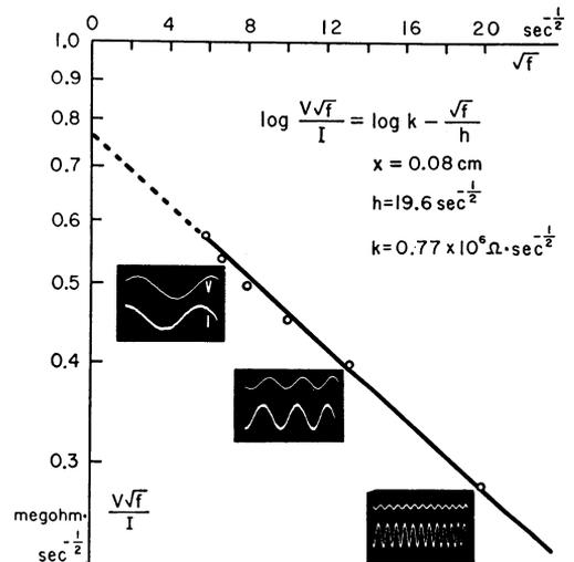
FIG. 4. Relationship among the amplitude of a sinusoidal current,  $I$ , sent into a muscle fiber at  $x = 0$ , the variation in the membrane potential,  $V$ , observed at  $x = 8$  mm and the frequency of the a.c.,  $f$ . The logarithm of  $V\sqrt{f}/I$  was plotted against  $\sqrt{f}$ . Further detail in text. 24°C.
