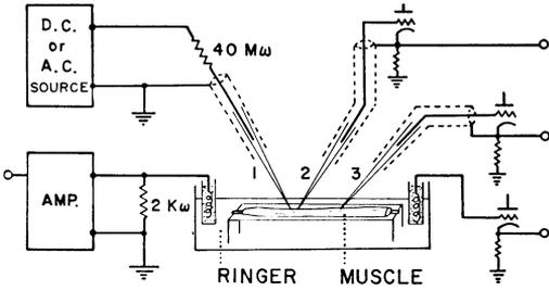
FIG. 1. Experimental arrangement used for determining the cable constants of a muscle fiber by the a.c. method and by the method based on the time constant of potential rise in the foot of a propagated action potential. Microelectrode #1 is for applying a d.c. pulse or a.c. to the muscle fiber, #2 and #3 for recording sinusoidal potential variations and action potentials. The large Ag-AgCl-agar electrode on the right in the diagram is the indifferent electrode for recording membrane potentials.
