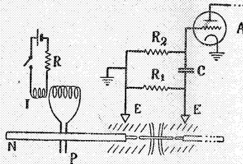
Fig. 1. Diagram showing the experimental arrangement. N, nerve; P, platinum electrodes; I, inductorium; R, resistance; R<sub>1</sub>, 50 (or 500), R<sub>2</sub>, 300 (or 500) kilo-ohms; C, condenser of 2 microfarads; E, non-polarizable electrode; A, amplifier.
