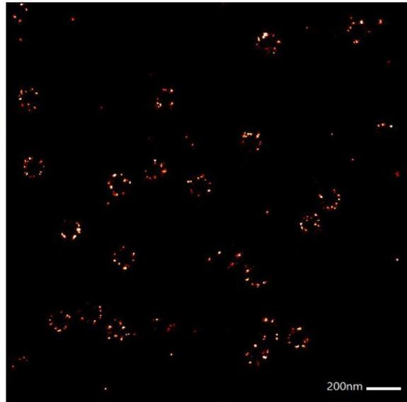
Comparative images of Nup96 complexes labelled with Alexa 647. Left: standard confocal mode, right: 2D Miniflux mode.
