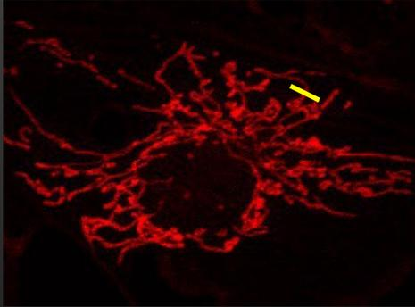
■ Noisy image = low signal (camera) or high gain (confocal PMT)
