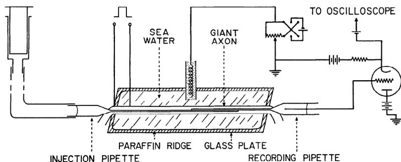
FIG. 1. Diagram of the injection apparatus.
