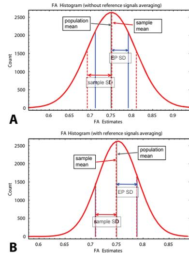
FIG 2. The FA histogram with sample SD and mean error-propagated (EP) SD of FA without reference-signal averaging (A), and with reference-signal averaging (B).
