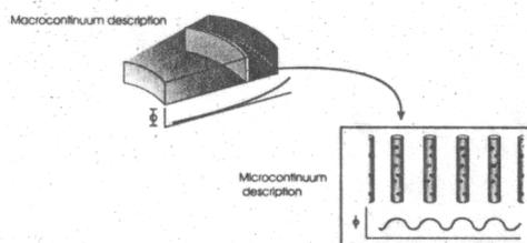
Fig 1: (a) macro- and (b) micro-continuum view of the solute and potential distributions in a centrifuge cell.
