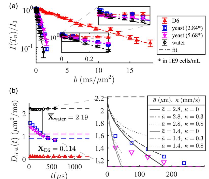
**Fig. 3:** Summary of results. (a) SG-TIETA decays plotted vs. the cumulative  $b$ -value for different experimental samples. (b) Inverted  $D_{\text{inst}}(t)$  curves. The yeast curves are compared to the theoretical short-time behavior [6] for mean pore size  $\bar{a}$  and permeability  $\kappa$ .
