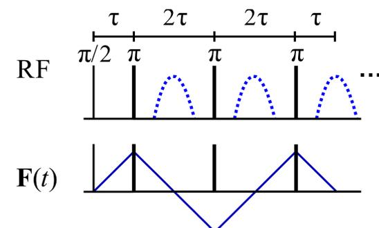
**Fig. 1:** Triangle wave  $\mathbf{F}(t)$  produced by the SG-CPMG sequence. The associated  $\mathbf{F}(\omega)$  focuses near  $\omega = 2\tau/\pi$  over many cycles.
