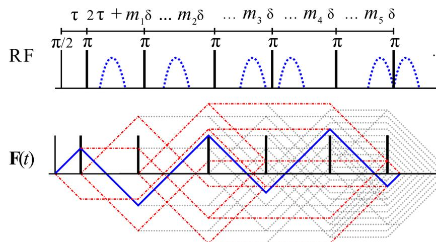
**Fig. 2:** Example SG-TIETA sequence with  $\tau = 4\delta$  and  $m_n = \{1, 3, 1, 2, 1\}$ . Various off-resonance CTPs which refocus (red, dashed) and do not refocus (gray, dotted) are shown.
